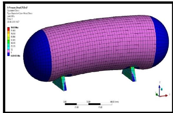
**Fig. 4. Equivalent stress for Al6082/5% ZrO<sub>2</sub> AMCs.**
