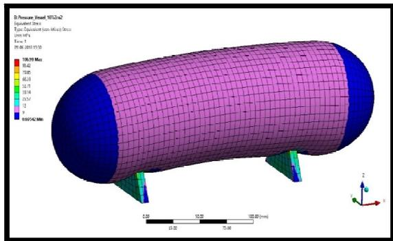
Fig. 5. Equivalent stress for Al6082/10% ZrO<sub>2</sub> AMCs.
