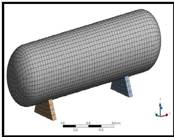
**Fig. 1. Meshed Pressure vessel.**
