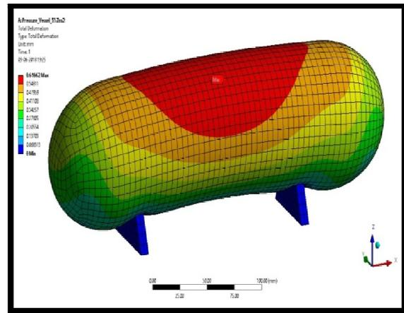
**Fig. 2. Total deformation for 0% Al6082 alloy.**
