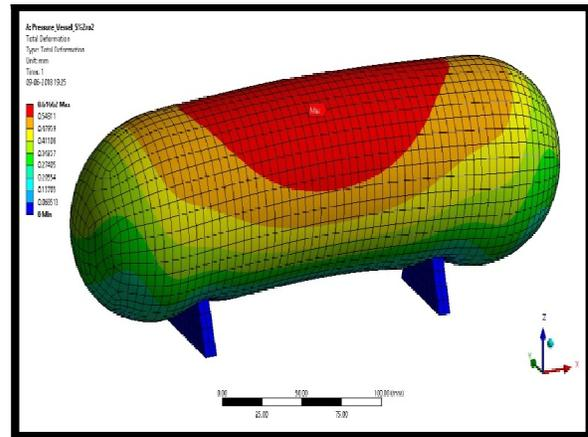
**Fig. 3. Total Deformation of Al6082/5% ZrO<sub>2</sub> AMCs.**
